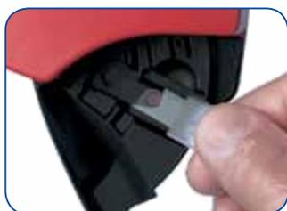
...place the filled microcuvette in the microcuvette holder and push the holder into the measuring position...
